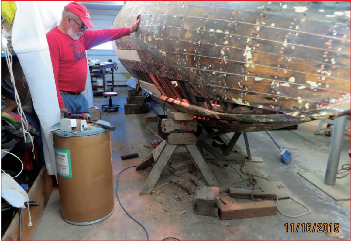
Refastening planking and plugging nail holes
